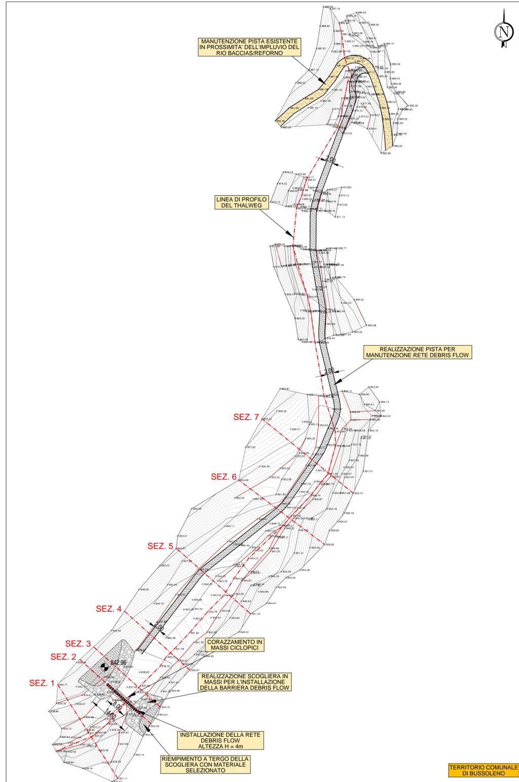
PLANIMETRIA DI PROGETTO - RETE DEBRIS FLOW
